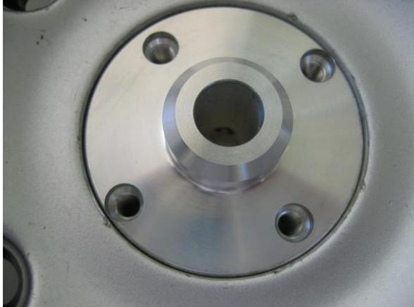
Looking at the non-drive side of the rear wheel with the adapter in place. Notice that there are two pairs of holes. Please use the pair that is closest to the edge of the wheel opening. In this case we will use the pair at the 2 and 8 o'clock positions.
