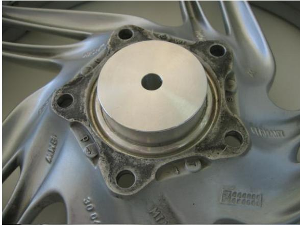
Slide the adapter in from the drive side of the rear wheel.
