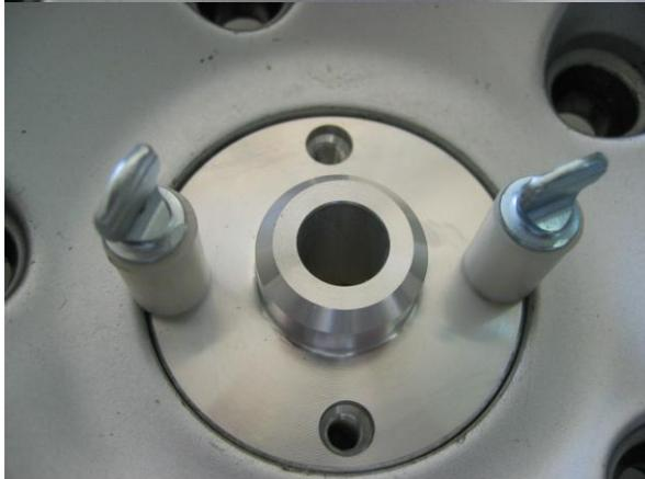
Slide the spacers onto the thumb screws and thread them into the adapter. They will hold the adapter securely in position. BMW wheel hubs have various thicknesses. Please choose the appropriate pair of spacers that will keep the thumb screws from bottoming in the adapter. Be sure to snug up the thumb screws evenly so as not to cock the adapter in the hole. You can now slide the axle through the adapter and suspend the assembly with the bearing blocks as normal.
