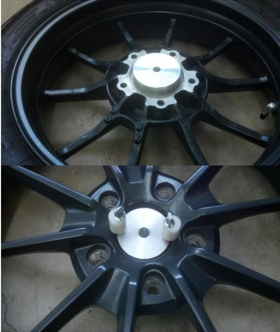
Slide the adapter in from the drive side of the rear wheel.
